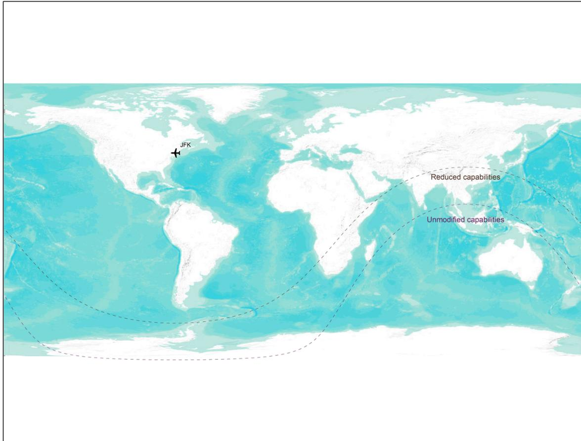
**Figure 2 Design range for the Boeing 787-8. Unmodified boundary as reported by Boeing. Reduced Capabilities is a 30% reduction in design range as modelled in Piano 5.**
