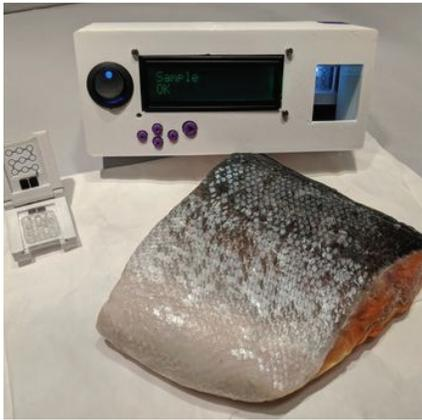
**FIGURE 5** A prototype Conservation X labs DNA scanner. These portable scanners could be used to identify seafood to species level and help to reduce seafood fraud. Credit: Conservation X
