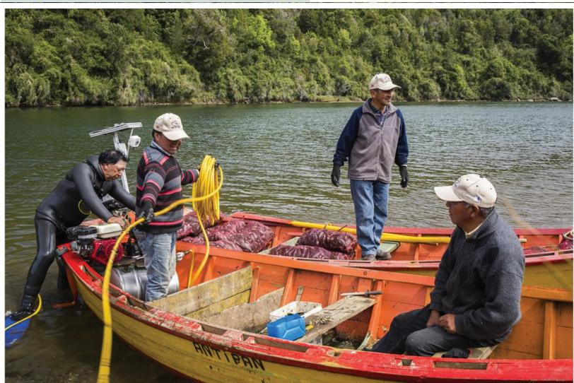
**FIGURE 2** A Shellcatch system installed on a small hookah diving vessel in Chile. Divers use an air compressor and a long air hose to allow them to harvest valuable benthic resources such as the loco (Concholepas concholepas) Credit: Marco Antonio
